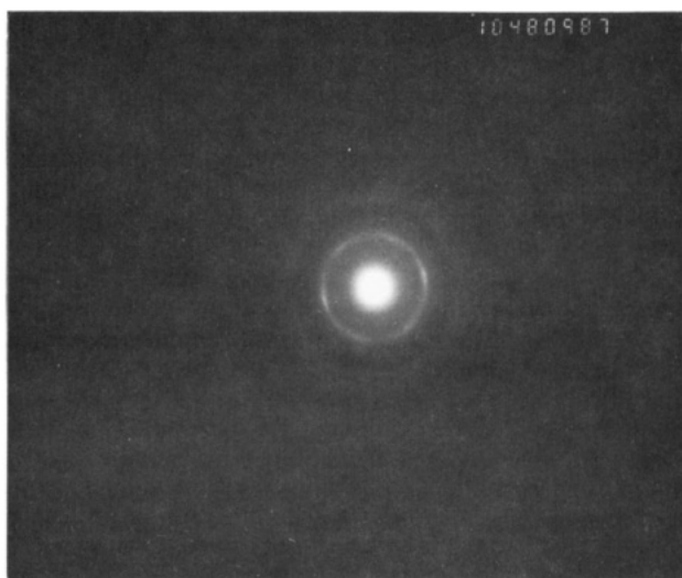
Figure 11. Electron diffraction pattern taken with the electron beam directed perpendicular to the platelet of sample \text{CdSe} \supset \text{Zr}(\text{O}_3\text{PCH}_2\text{CH}_2\text{CO}_2\text{H})_2 .
